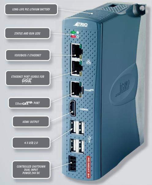
Trio's PC-MCAT 64 is an innovative "Motion + PC Solution". A powerful quad core Intel Atom processor is used to drive both a high performance motion controller and a compact PC that can run user applications under Windows. The PC-MCAT software uses a real-time extension to allow both Windows and the motion controller to run directly on their own processor cores.
